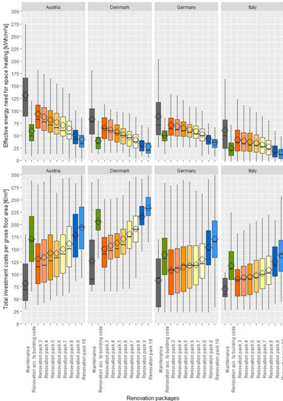
Figure 3: Box plots of effective energy needs and total investment costs for all building classes in the different countries when implementing the maintenance and renovation packages as defined for this analysis
